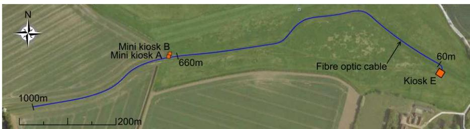
Figure 2. Fibre optic cable configuration with distance markings according to the distance reported by the DTS unit
