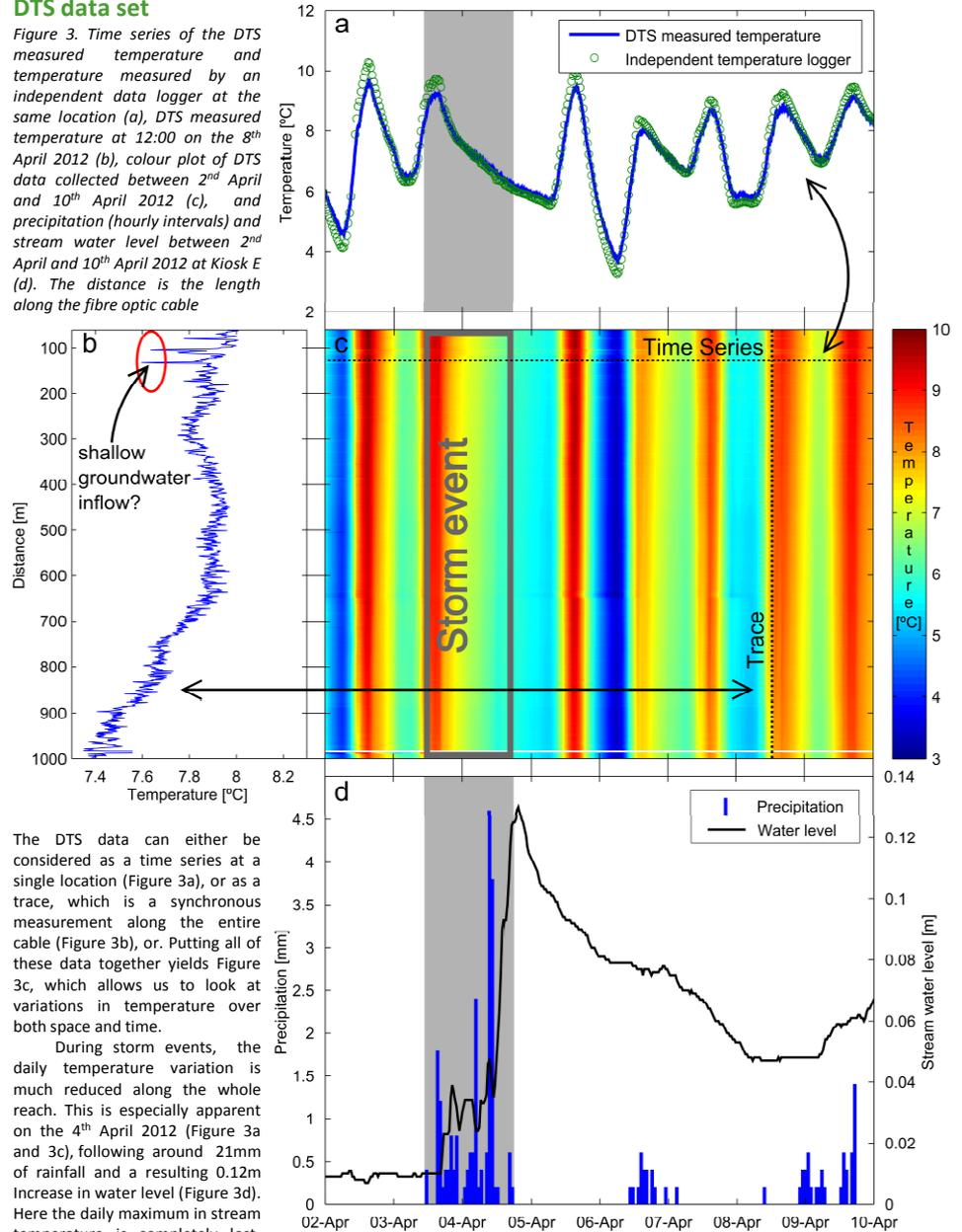
The DTS data can either be considered as a time series at a single location (Figure 3a), or as a trace, which is a synchronous measurement along the entire cable (Figure 3b), or. Putting all of these data together yields Figure 3c, which allows us to look at variations in temperature over both space and time.
