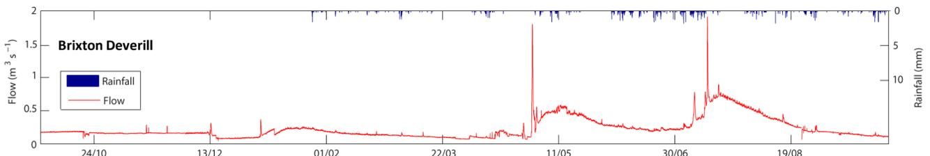
Figure 2: Plots showing example rainfall and discharge data for the Brixton Deverill field site during the Water Year 2011-2012 (Oct 2011 – Sept 2012).
